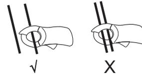
**Note:** The clamp jaws must be fully closed for proper measurements. On large conductors or line splitters, make sure there is no gap between the upper and lower jaw.
