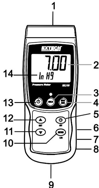
**Notes:** Items 6, 7, and 8 are located behind the snap-off compartment cover on meter's right side. Battery compartment, tilt stand, and tripod mount are located on the rear of the instrument
